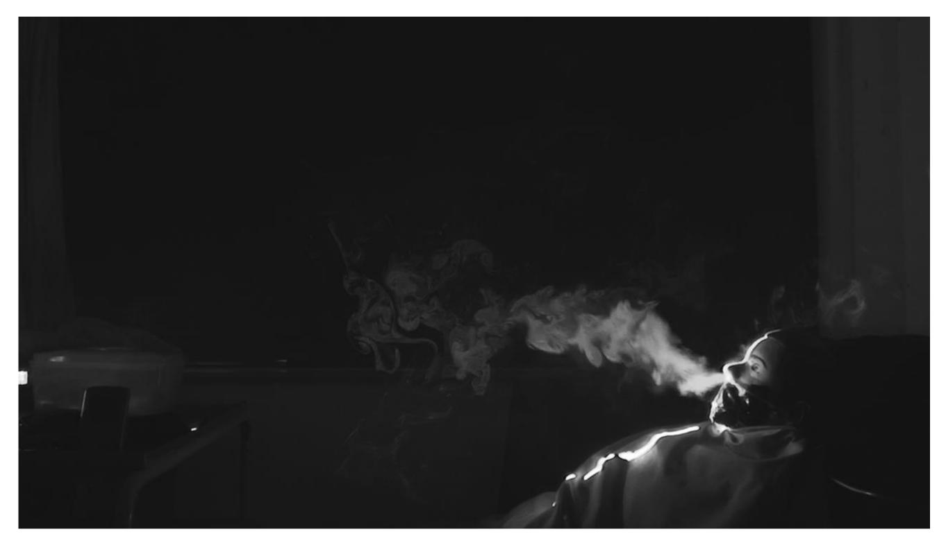
Figure: Grey scale camera frames captured for light intensity analysis routine to generate normalized particle concentration contours.
